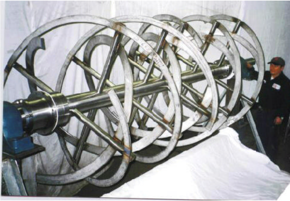
Impeller for Ribbon Blender, double flight, ends discharge.
