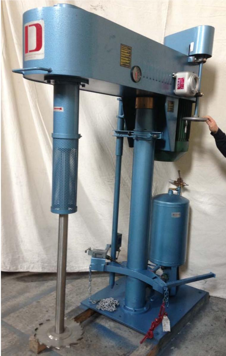
Series 2010 Dispersers are offered in standard motors horsepower from 3 to 100 HP.
