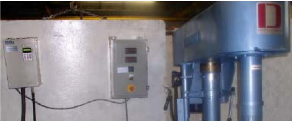
The Controller in NEMA 1 enclosure is shown on the left. The Remote Control Box is shown in the center. The Controller may be mounted in power room. The Remote Control Box may be mounted on the Disperser or on the wall, wherever convenient. These models are also available with explosion proof motors and remote control box.
