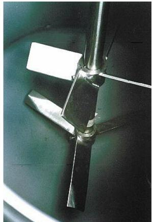
REACTOR, SANITARY FINISH, VACUUM/PRESSURE, F&D BOTTOM & TOP, HEATING JACKET 75 PSIG & 350 DEGREES F, VARIABLE LOW SPEED AGITATOR, HIGH EFFICIENCY BOTTOM TURBINE
